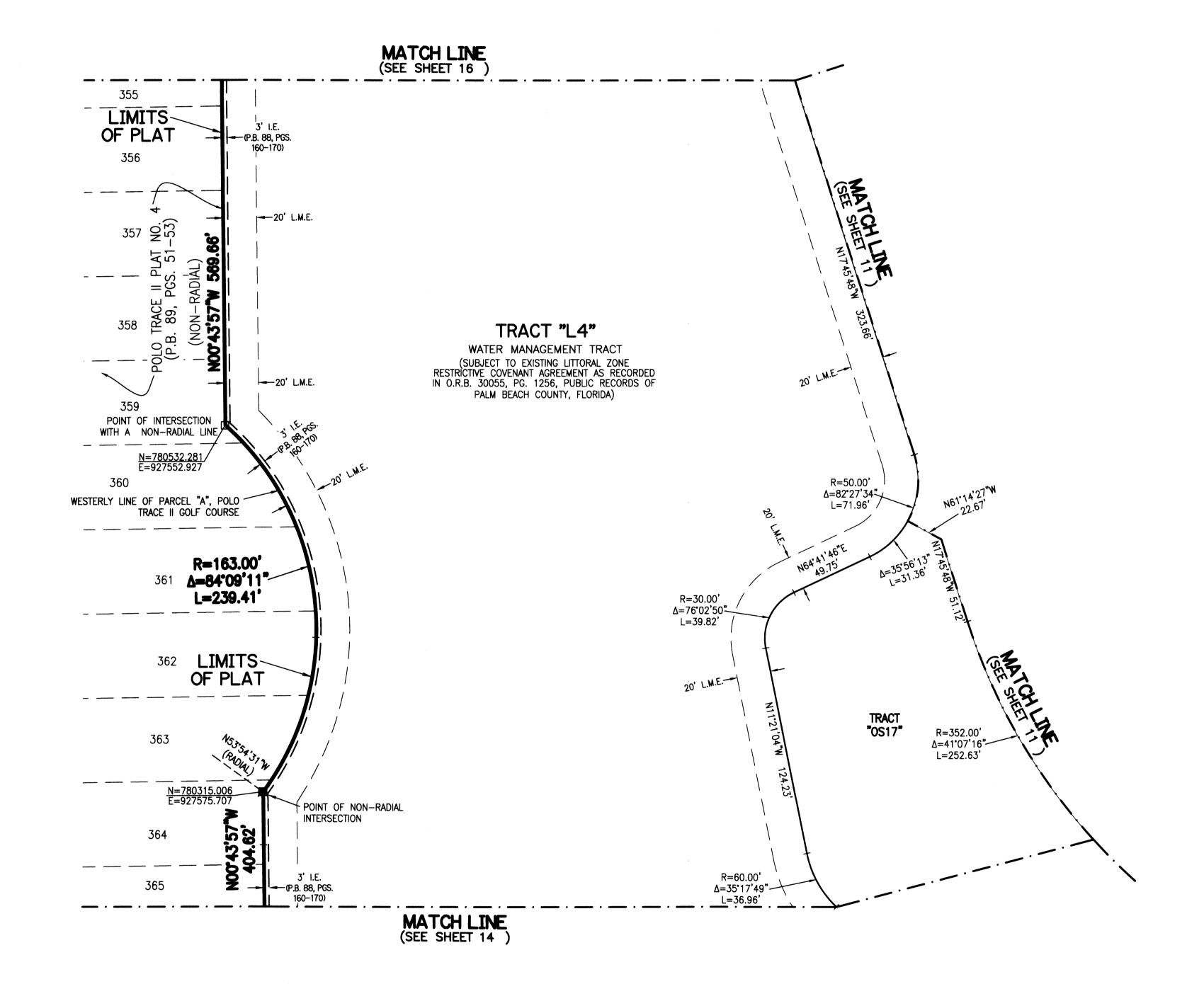
COORDINATES SHOWN ARE GRID COORDINATES DATUM = NAD 83 (1990 ADJUSTMENT) ZONE = FLORIDA EAST ZONE LINEAR UNIT = U.S. SURVEY FEET COORDINATE SYSTEM = 1983 STATE PLANE TRANSVERSE MERCATOR PROJECTION ALL DISTANCES ARE GROUND SCALE FACTOR = 1.0000258PLAT BEARING = GRID BEARING GROUND DISTANCE X SCALE FACTOR = GRID DISTANCE
